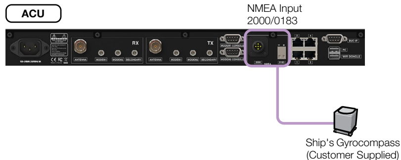
Figure 28: Ship's Gyrocompass Cable Connection
