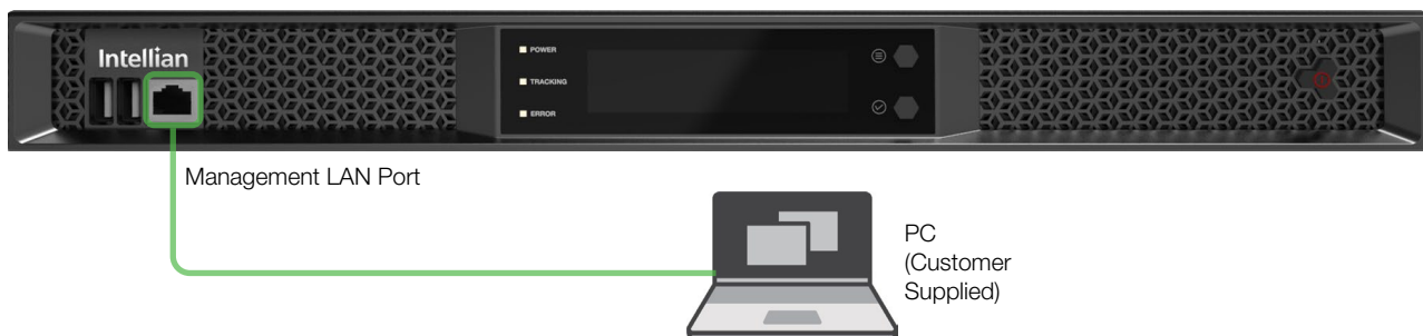
Figure 32: Front Panel Management LAN Port Connection
