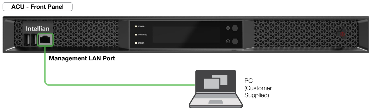
Figure 30: Front Panel Management LAN Port Connection
