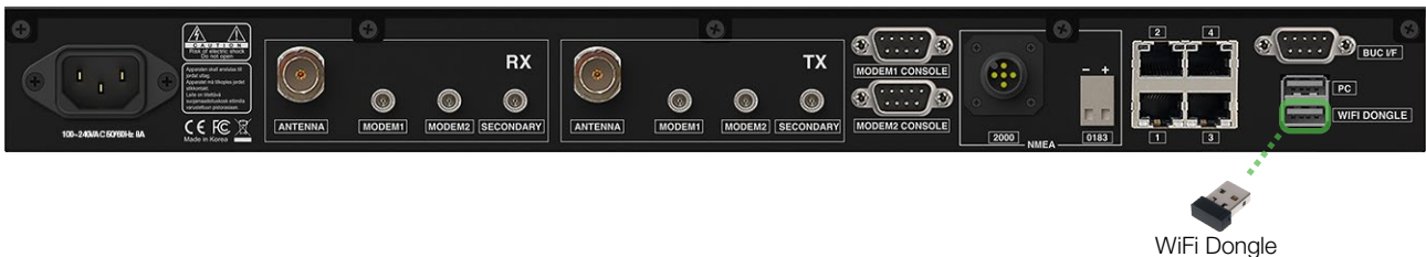
Figure 31: Back Panel Wi-Fi Dongle Connection
