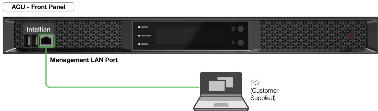
Figure 32: Front Panel Management LAN Port Connection
