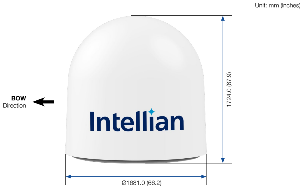
Figure 7: Antenna Side View
