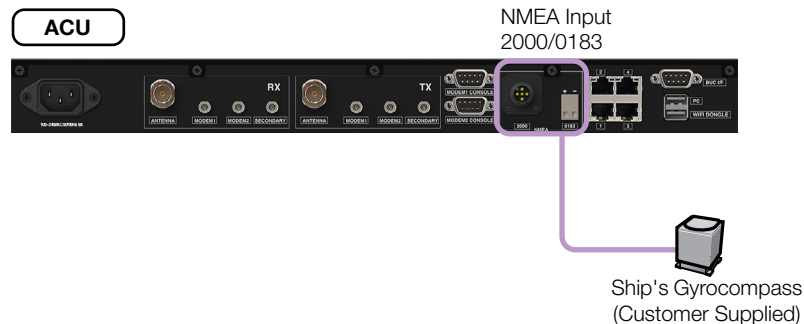
Figure 30: Ship's Gyrocompass Cable Connection
