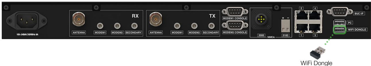
Figure 33: Back Panel Wi-Fi Dongle Connection
