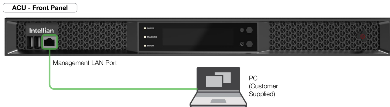
Figure 35: Front Panel Management LAN Port Connection
