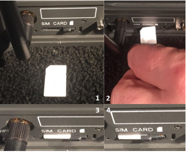
Installing SIM card and engaging the lock
