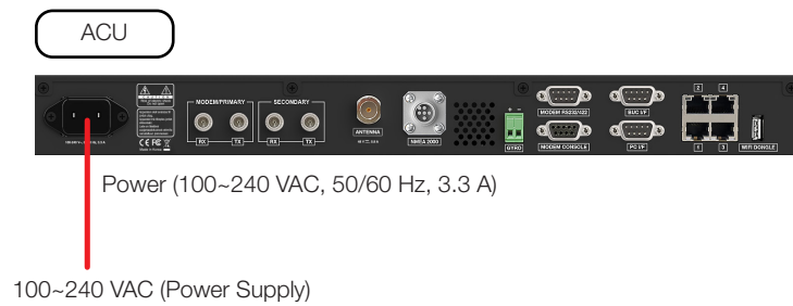
Figure 22: Connecting Power to ACU
