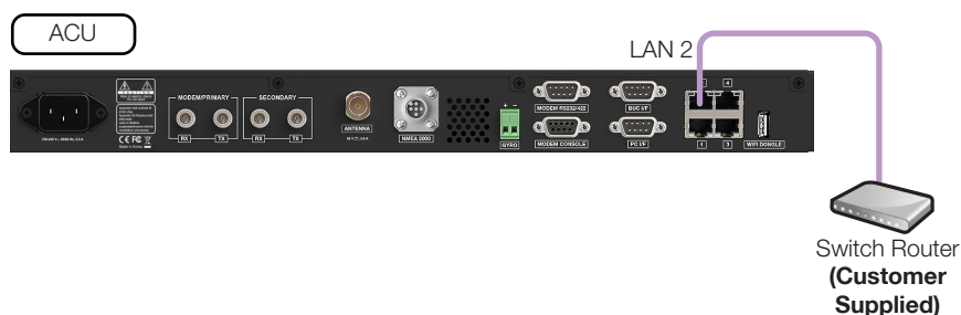
Figure 27: ACU to Switch Router Cable Connection
