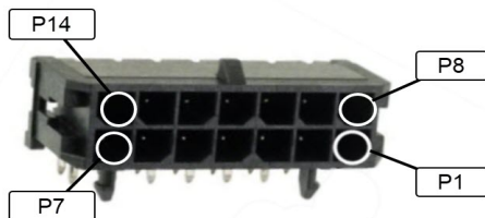
Figure 1-2. SMB3315 Power and Status Connector Pin Locations
