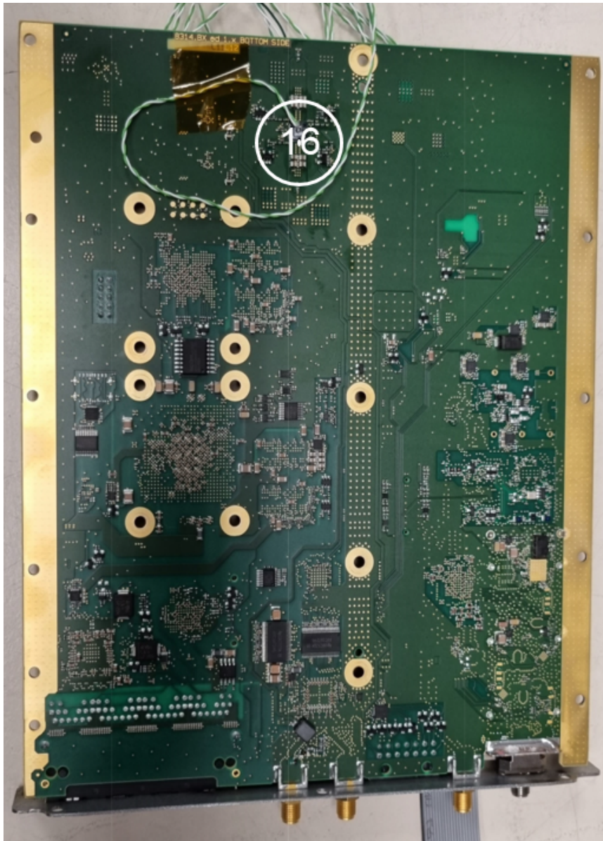
Figure 1-7. Locations of Recorded Case Temperatures - Bottom Side of Board
