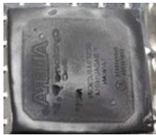
Figure 1-8. Example of Pad Local Deformation and Compression
