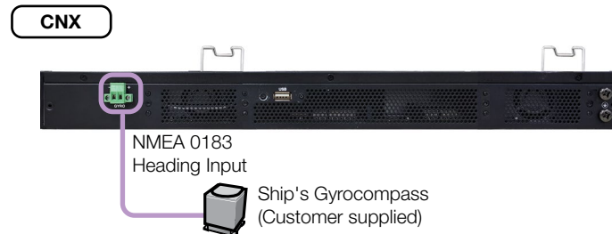
Figure 22: Ship's Gyrocompass Cable Connection
