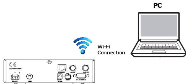
Figure 27 : ACU to PC Wifi Connection
