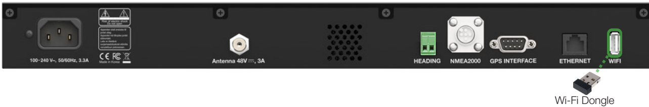
Figure 31: Rear Panel Wi-Fi Dongle Connection
