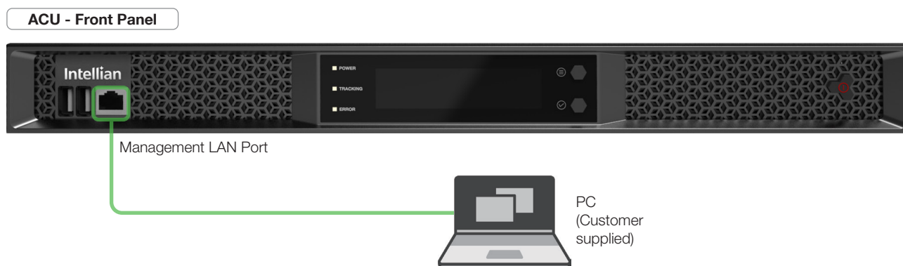
Figure 32: Front Panel Management LAN Port Connection
