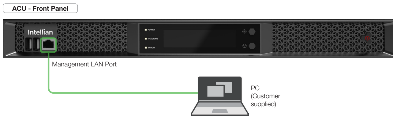
Figure 30: Front Panel Management LAN Port Connection
