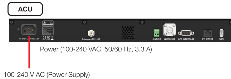
Figure 22: Connecting Power to ACU
