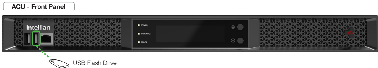
Figure 28: Front Panel USB Port Connection
