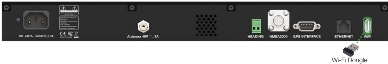
Figure 29: Rear Panel Wi-Fi Dongle Connection
