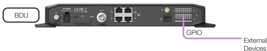
Figure 43: BDU to External Devices Connection
