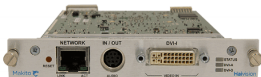
Sample Rear View (DVI Blade #B-292E-DVI)
