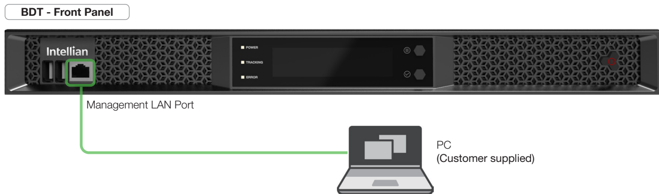
Figure 32: Front Panel Management LAN Port Connection
