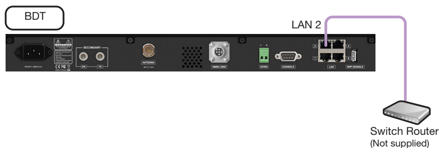
Figure 28: BDU to Switch Router Cable Connection
