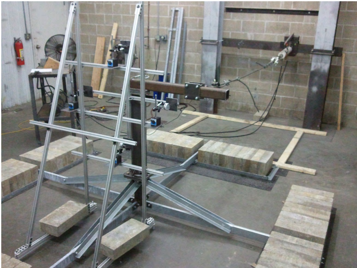
*B6-116 KA non-penetrating mount with four (4) gauges set to collect measurements for total angular deflection.
