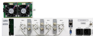
Hot-swap power supplies, forced air cooling trays and amplifier modules (rear panel view of similar model)
