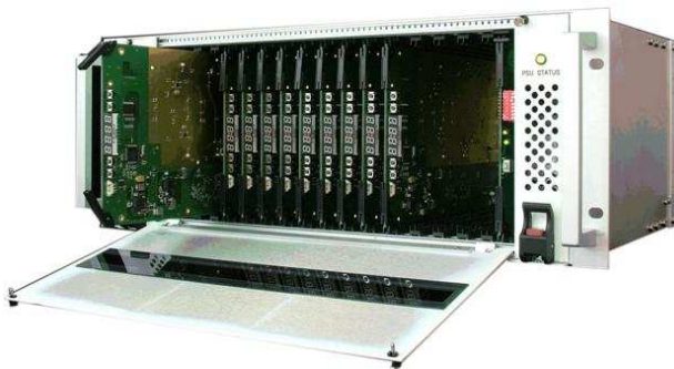
Front view showing hot-swap RF Module
